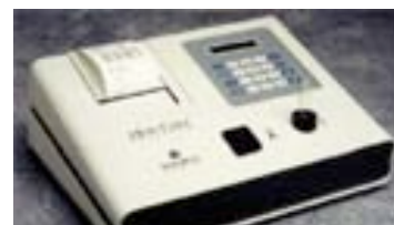
Figure 7. This point-of-care instrument is a multiple wavelength spectrophotometer with an integrated printer for patient results.
