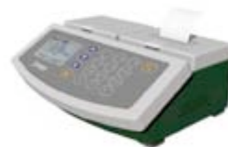
Figure 2. This POC instrument was developed for testing food toxins using fluorescence detection. The instrument was based on a low-cost 68HC12 microprocessor platform.
