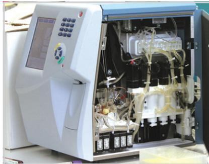
**Figure 1.** Comprised of pumps, motors, syringes, tubing, optics, electronics, and software, this hematology analyzer, developed and manufactured by BIT C2 Diagnostics, performs an intricate and delicate task. Multidisciplinary skills in mechanics, chemistry, electronics, software, optics, and fluidics are necessary to engineer and develop such an instrument.
