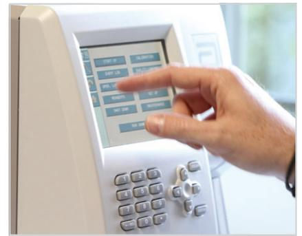
**Figure 4.** The graphical user interface (GUI) provides menus with selections used by the administrator of the instrument to control the underlying processes. The graphical menus serve to enrich the user experience and help to reduce operator error.
